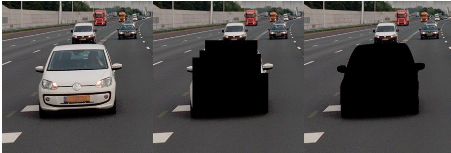
Figure 26. Left: Unmasked image crop; note that private information was blurred manually for publication. Middle: Image masked based on Cyclomedia segmentation. Right: Image masked based on refined mask, generated with SAM (Kirillov et al., 2023).
