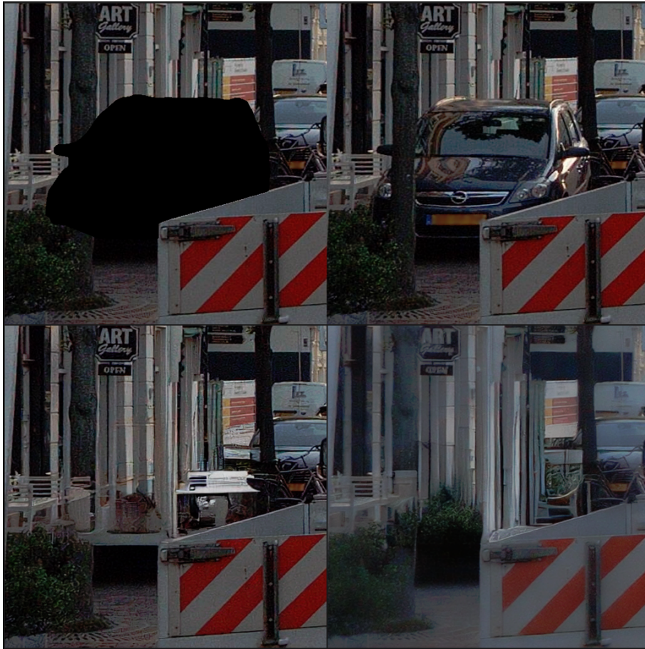
Figure 33. Top left: Masked image, mask was drawn by hand for testing purposes. Top right: Original image. Bottom left: Baseline model output. Bottom right: Unweighted Partial Loss model output. Note that the license plates were manually blurred for publication.
