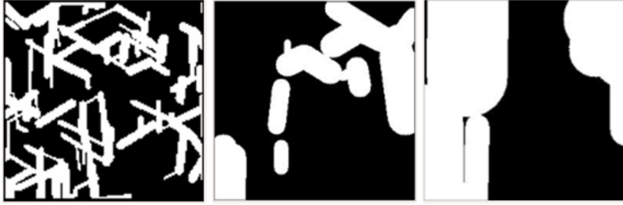
Figure 23. Different types of polygonal synthetic masks generated following the Suvorov et al. (2021) method. Left: Thin mask. Middle: Medium mask. Right: Thick mask.
