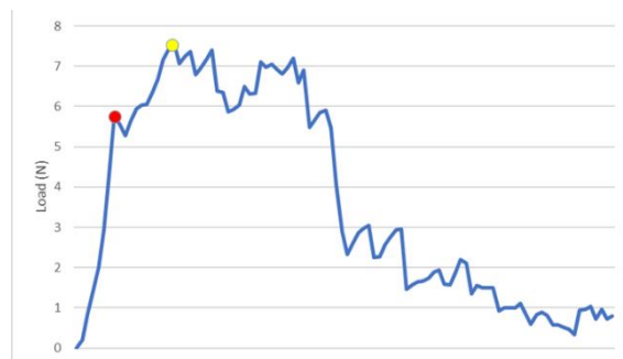
Figure 2. Results generated by the Instron of the material tests. Yellow dot representing the plasticity barrier, red dot representing the maximum load the material could carry.
