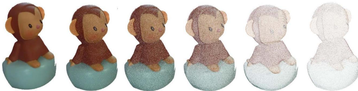
Figure 12 Monkey point cloud models in different resolution by down-sample (Zhang et al, 2014)
