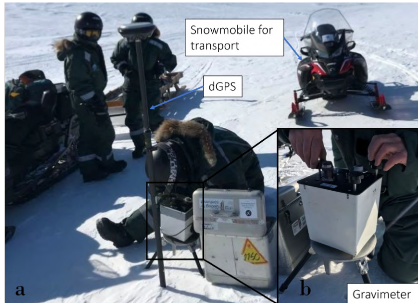
Figure 4.4: Figure illustrating the acquisition of gravity data in the field during the 2022 survey. a) The closest instrument is a Leica Viva GS16 dGPS used for accurate positioning in the field. The LaCoste & Romberg gravimeter is placed on a tripod behind it. b) The tripod is used to bring the gravimeter to a completely horizontal level, after which the relative gravity value could be determined. Figure adapted from Rylander & Sterley (2022).
