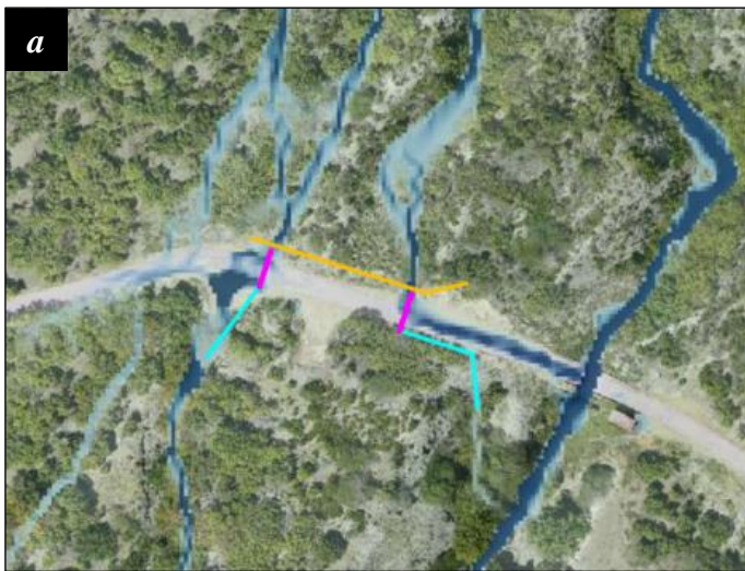
Figure 6.4: Possible drainage layouts for the active gullies. a. Two new culverts below Weg near White Wall for gully 2 and gully 3. A retaining wall at the upstream side should prevent runoff from circumventing the culvert. Protected outlets guide the runoff towards the downslope gully sections; b. Rerouting towards gully 1. A retaining wall concentrates the runoff towards channels that guide the water to the culvert of gully 1. These maps are included on a larger size in APPENDIX 4.
