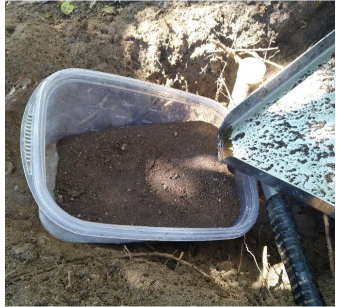
Figure 5.3: Water beading up on the soil in the runoff collection pit (left); soil particles staying afloat in a runoff collection container (right).
