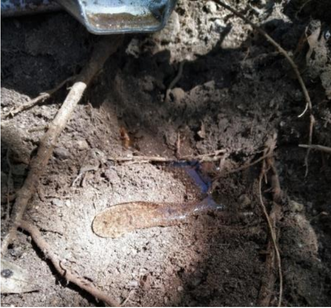
Figure 5.3: Water beading up on the soil in the runoff collection pit (left); soil particles staying afloat in a runoff collection container (right).
