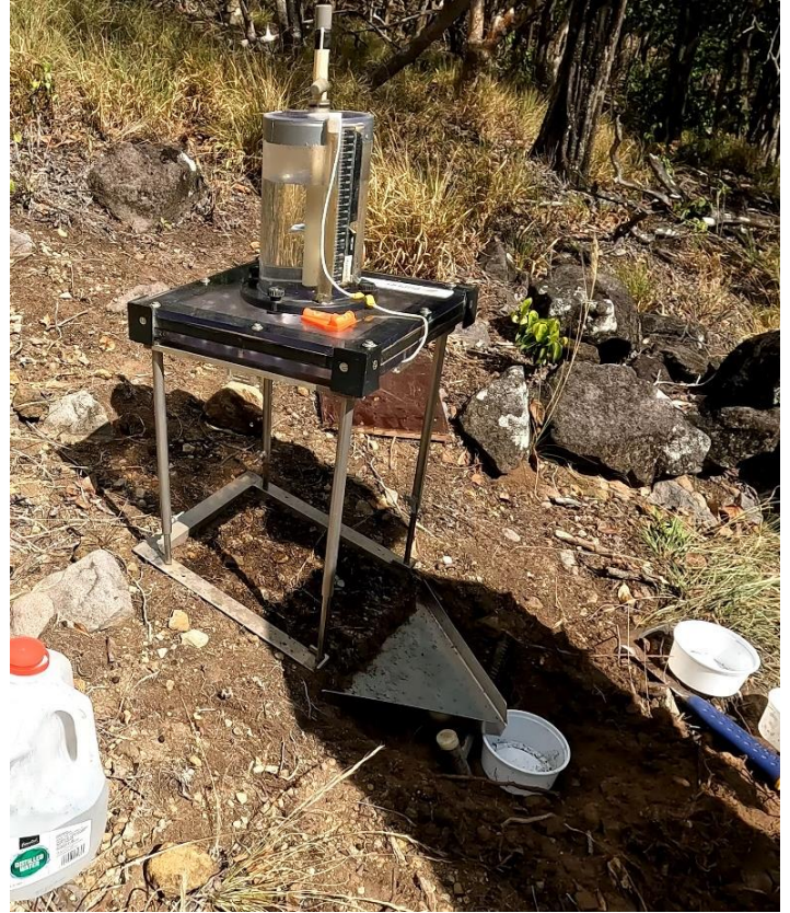
Figure 4.3: Schematic setup of the rainfall simulator, adapted from the instructions by Eijkelkamp (left); The rainfall simulator set up in the field (right). Over the course of the experiment, the hydraulic head in the reservoir remains constant, ensuring a steady input of water. Water drips through the perforations and is guided downslope via a trough into a collection container. At set intervals, the discharge from the reservoir and the runoff in the container are measured.
