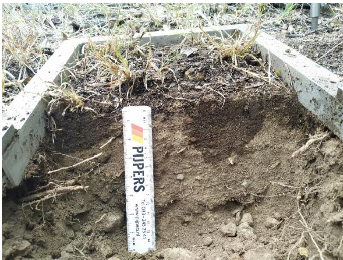
Figure 5.4: Preferential flow paths in a soil with low permeability (left). Besides the flow paths, infiltration in this soil was very limited; Uniform infiltration in a soil with high permeability (right).
