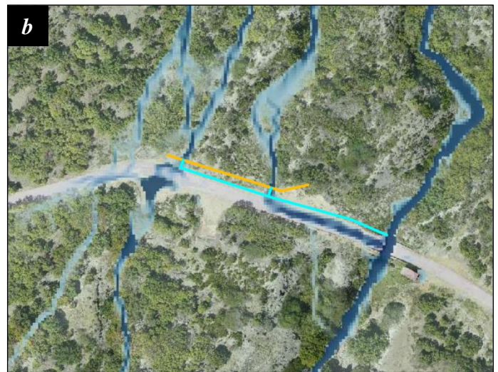
Figure 6.4: Possible drainage layouts for the active gullies. a. Two new culverts below Weg near White Wall for gully 2 and gully 3. A retaining wall at the upstream side should prevent runoff from circumventing the culvert. Protected outlets guide the runoff towards the downslope gully sections; b. Rerouting towards gully 1. A retaining wall concentrates the runoff towards channels that guide the water to the culvert of gully 1. These maps are included on a larger size in APPENDIX 4.
