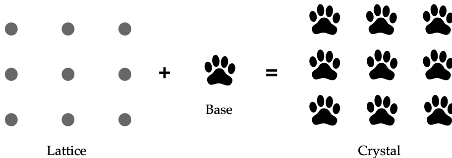
Figure 3.1: Representative example of a crystal: to each site on a lattice, a generic and purely illustrative basis is attached to form a crystal structure.
