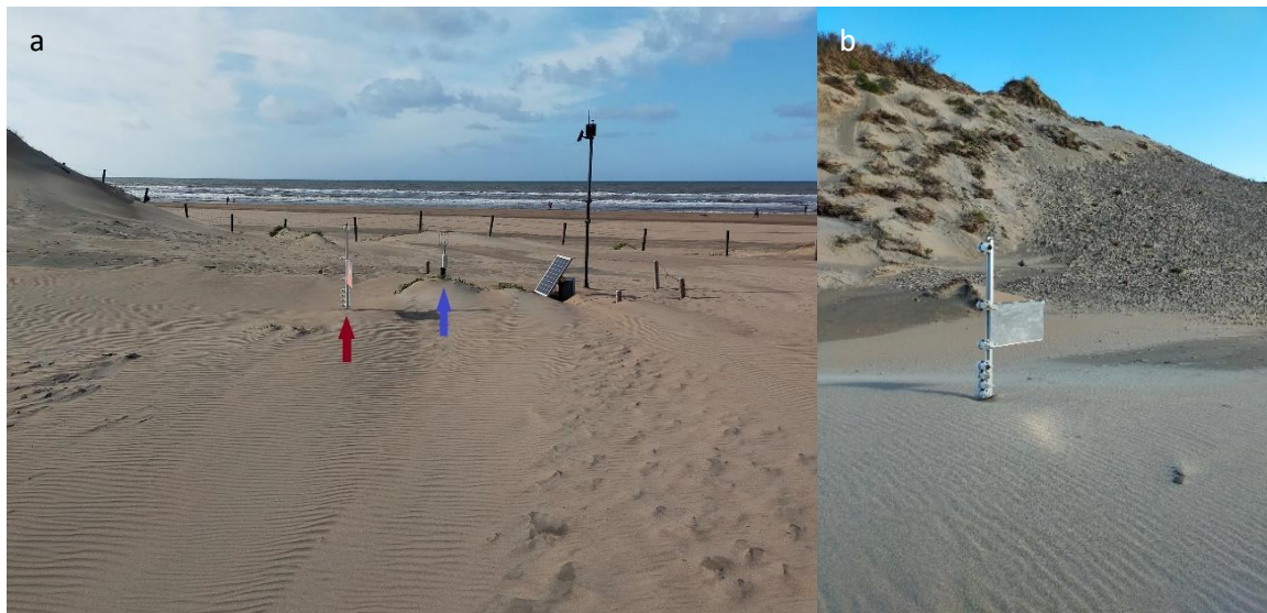
Figure 4: a) Sand catcher (indicated by the red arrow) next to the most seaward ultrasonic anemometer (blue arrow). b) Close up of a sand catcher, in the background the northern wall is visible. Both pictures are taken at 16 Oct '22
