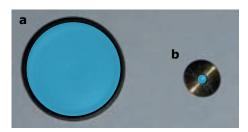
Figure 3.1: The a) large and b) small sample holders used for measurements. The blue circles indicate the placement of sample material.
