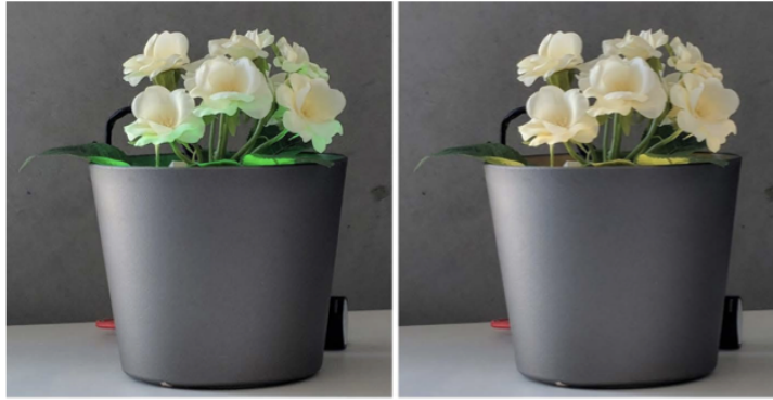
FIGURE 2.6: Smart Plant System , Müller et al., a persistent display hidden in a plant pot.
