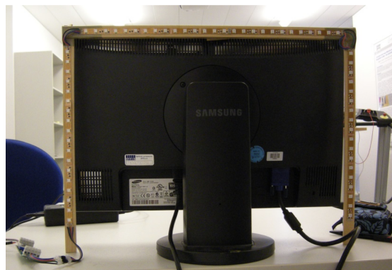
FIGURE 2.5: Ambient Timer , Müller et al. LED-Frame mounted on the backside of the monitor.
