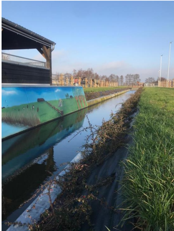
Figure 2. Overview of the water track used in this study. The water height was set on 33 centimeters and the track has a length of 85 meters.
