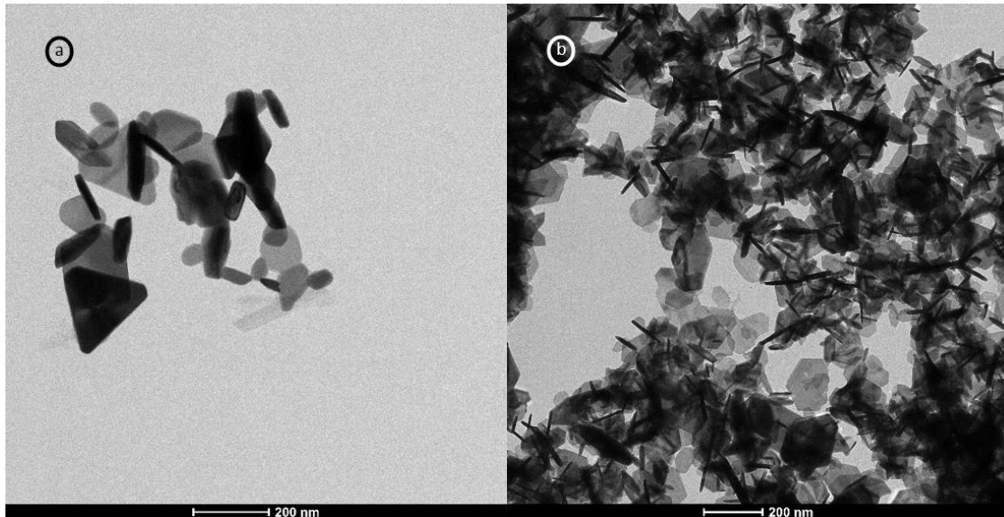
Figure 4.15: Representative TEM images of \text{Bi}_2\text{Se}_3 NPLs obtained by polyol hot injection procedure at varying surfactant concentrations. a) No PVP, b) OLAM instead of PVP.
