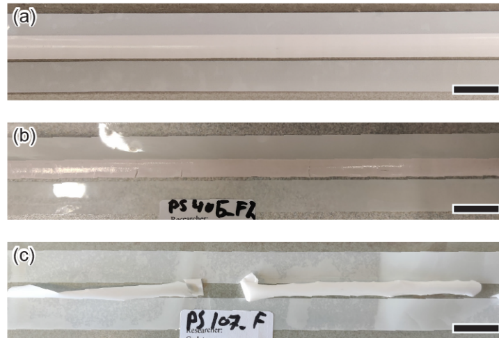
Figure 4.2: Poly-BDA membranes that have (a) stayed intact, (b) cracked, and (c) curled up during drying. Scale bar is 20 mm.
