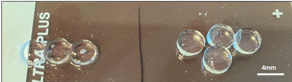
Figure 12: 6.1.3 Hydrogel casting – Comparison of the GelNOR discs before (left) and after the second dialysis (right). The hydrogels were casted in with a GelNOR concentration of 10% w/v, containing 0.05% w/v LAP and 10mM DTT in an UV-oven for 10 minutes ( \lambda = 365 \text{ nm} ).
