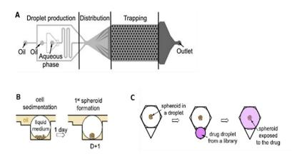
*Figure 2. Overview microfluidic chip design. A.* Composition of chip from injection to outlet region. *B.* Spheroid formation after injection of liquid medium containing cells. *C.* Drug screening with fluorescent second droplets. Pictures adapted and retrieved from <sup>15</sup>.
