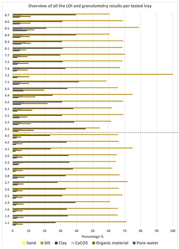
*Figure 27: Overview of all the LOI and granulometry results per tested tray with dashed line split between provinces.*
