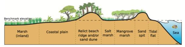
*Figure 3: Schematic profile of the coastal provinces in the Mekong Delta. Adapted from (Minderhoud, 2019).*
