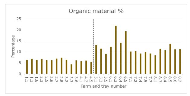
*Figure 23: Organic material percentage in the LOI tested sediments with dashed line split between provinces.*
