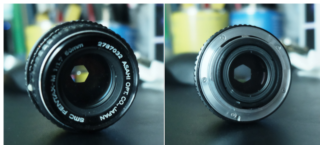
Figure 2.6: The entrance pupil (on the left) and exit pupil (on the right).
