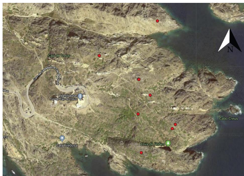
Figure 7.3 Ground control points (GCPs) for the Lighthouse Area are used for accurate Georeferencing of the obtained photogrammetric model and orthophotos. GCPs are placed at different heights relative to the take-off point to reduce 3D distortion—the road for scale.
