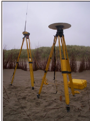
Picture 2-2 Base station of DGPS with the radio station at the left side and receiver at the right side.
