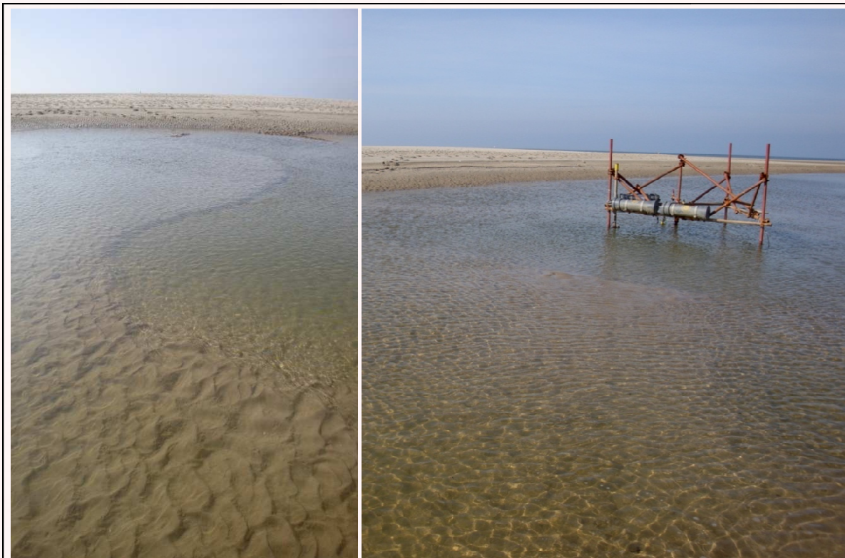
Picture 4-1 Dune formations in the Sluifers main channel. A) Lateral distribution of dune crest following a point shaped line, picture was taken on September 25, 2008 at 11:02. B) Sharp transition of bed level near the measuring frame.
