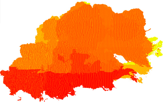
(c) Shaded by index into the voxel index. Shown is a conversion from index to hue using the following formula: x + y \times dim\_size + z \times dim\_size^2 . The striped pattern is a result of bricks ( 8^3 voxels) are a combination of two texture slices, these are the altering index colors. The larger shifts in color, which are in specific cubic regions, correlate to the different L2 nodes.
