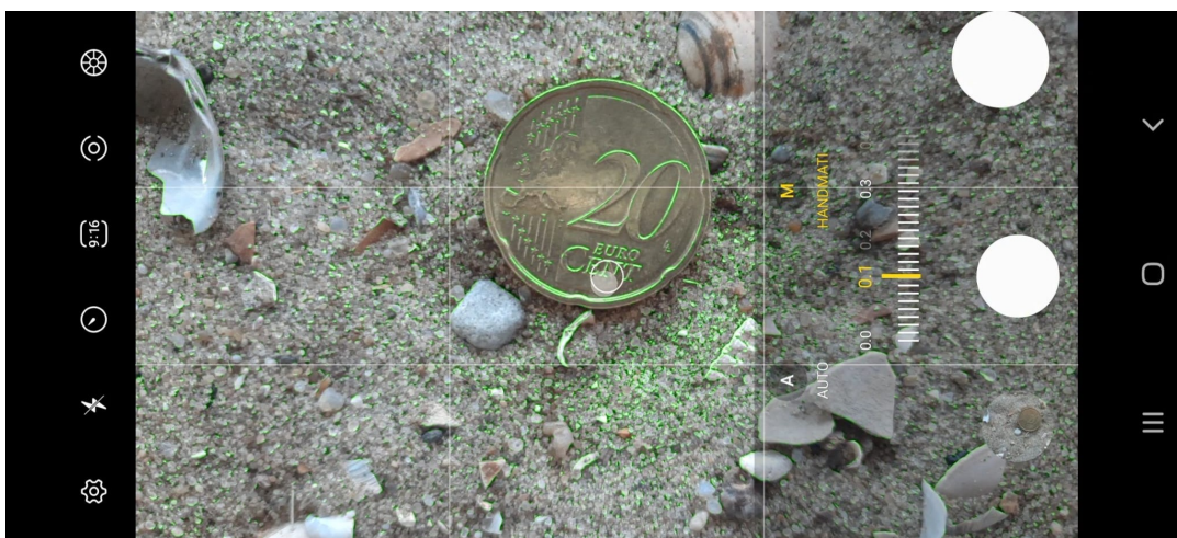
Figure 3.4: Screenshot from default camera application of the Samsung Galaxy A51, using manual focus. The light-green colour visible in the image is an added edge-detection filter.
