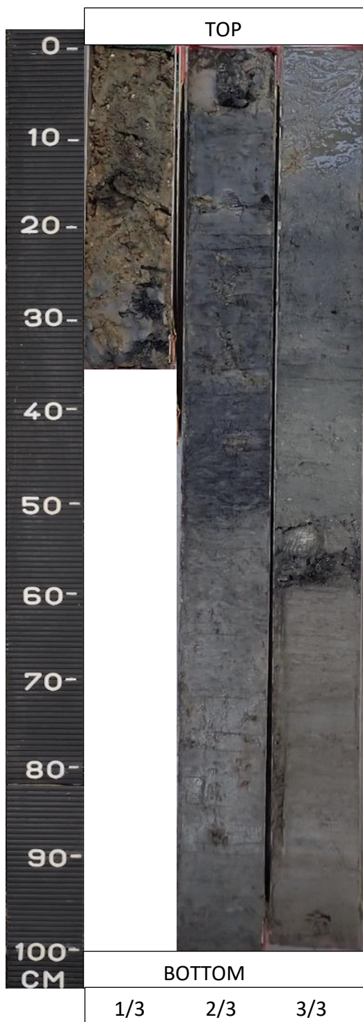
Core photographs of borehole SS22-320-VC14 (Brown Bank Member): interval of 8-233 cmbs. Photo courtesy of TNO geological survey of the Netherlands.
