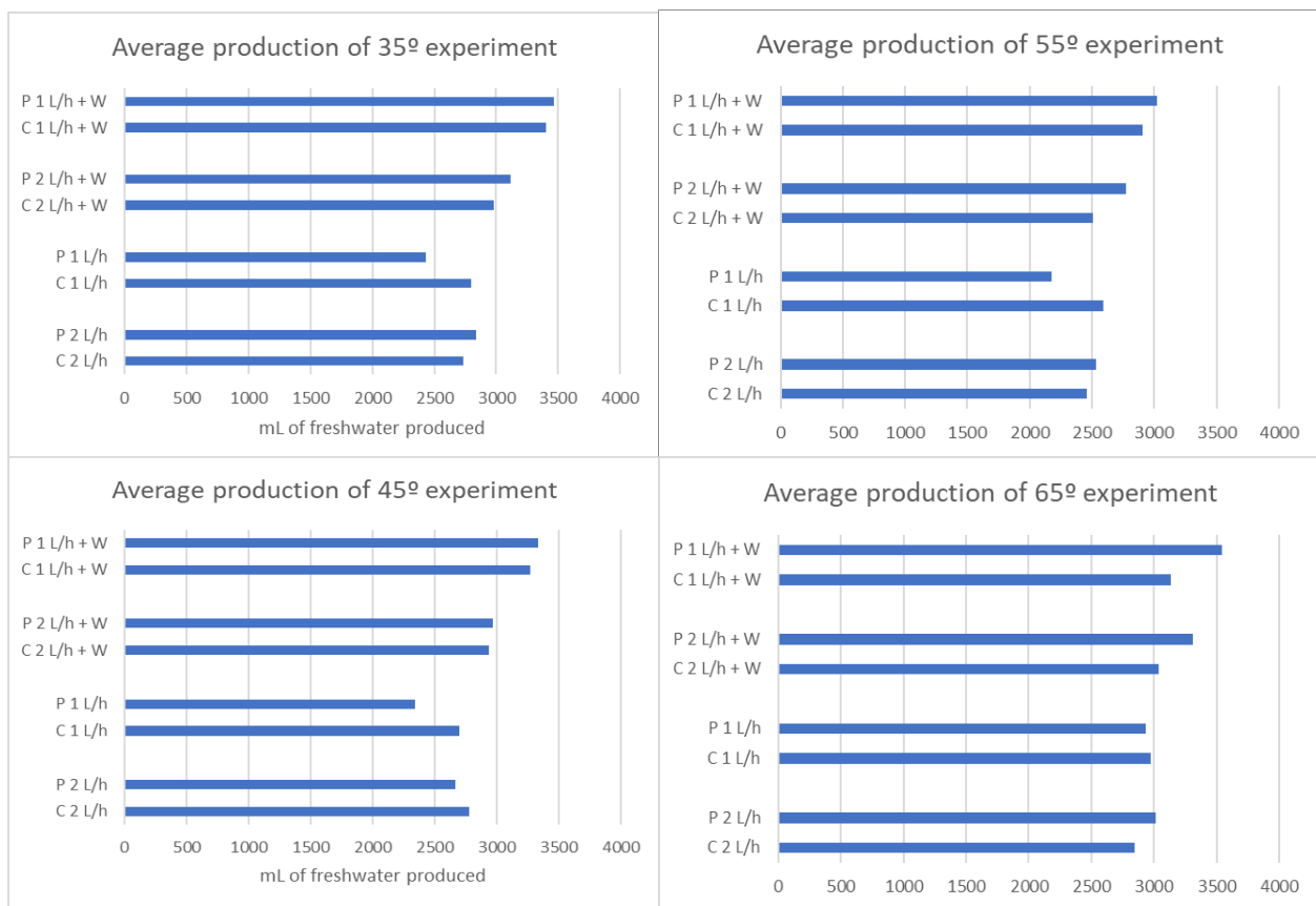
Figure X. Average water production in each experiment. 'P' stands for preheated, while 'C' for control. 'W' indicates the presence of wick material.
