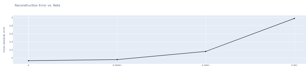
Figure C.7: Reconstruction accuracy of \beta -VAE models with 6 latent units, at different values of \beta . Values on the x-axis indicate the \beta value that was used. Larger \beta values result in a worsening of the reconstruction quality.
