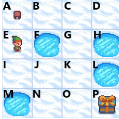
► Figure 6.1: Example environment of a reinforcement learning task: the OpenAI gym “Frozen lake” task, where the player (the elf) should move across the ice from its stool to the gift, without falling into any of the holes in the ice.
