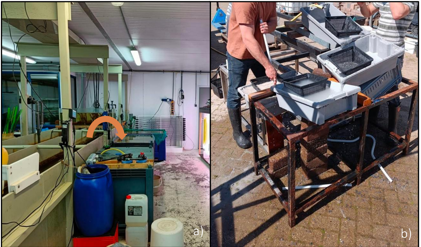
Figure 5. Pictures depicting the initial procedures for the set-up of the tank. a) the orange arrow shows the movement of the waste produced in the system into the container where the microbiota was being grown. b) the process of washing the gravel.
