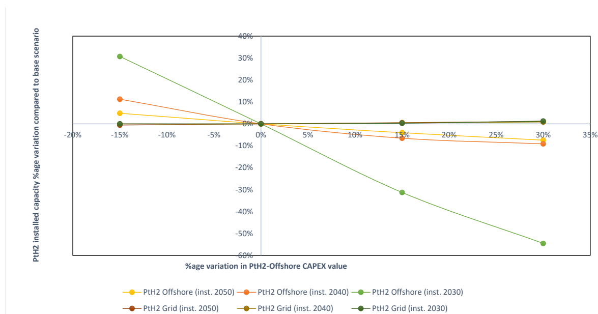
Figure 4.15: Installed capacity sensitivity of offshore and onshore electrolyser (PtH2) as a function of offshore electrolyser CAPEX variations
