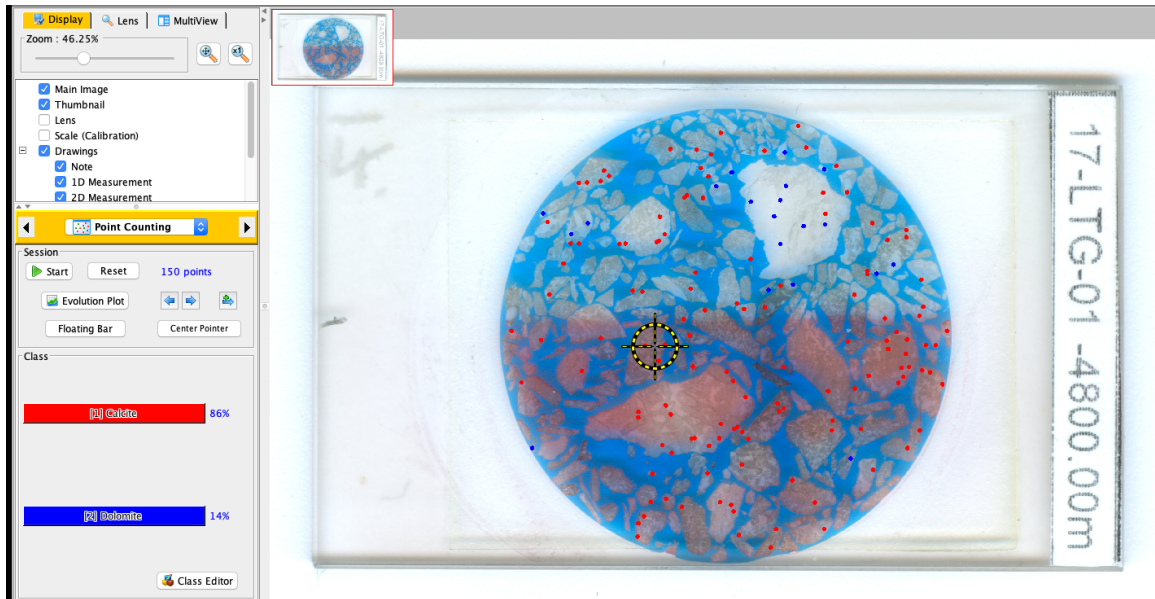
Figure 45: Cuttings point counting on sample 17-LTG-01 (depth: 4800m). Results are shown in the bottom left corner.
