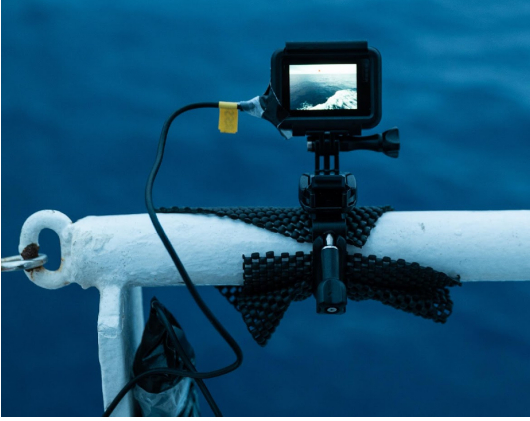
(a) Ship-Based Camera Set-up: A GoPro® Hero6 Black clamped to the ship starboard and/or port-side railing.
