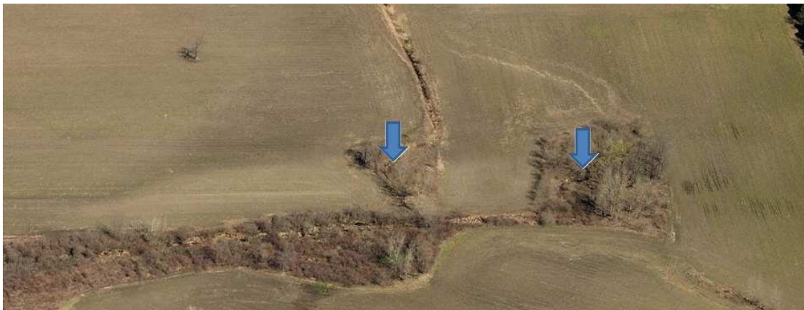
Figure 4.5 Photograph of the flood zone in the Quinlan road watershed. The blue arrows show the locations of the sinkholes. Darker colouring of the soil indicates higher soil moisture content and is related to local depressions (source: Microsoft Windows Live Maps).
