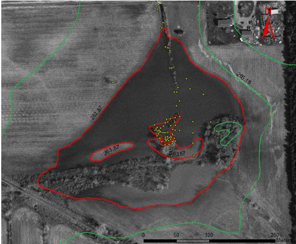
Figure 4.6a Aerial photograph showing the extent of the 2005 flood event. Green contour lines are extracted from a topographic map. Additional contour lines are shown in red. Height measurements coming from survey data are yellow dots.
