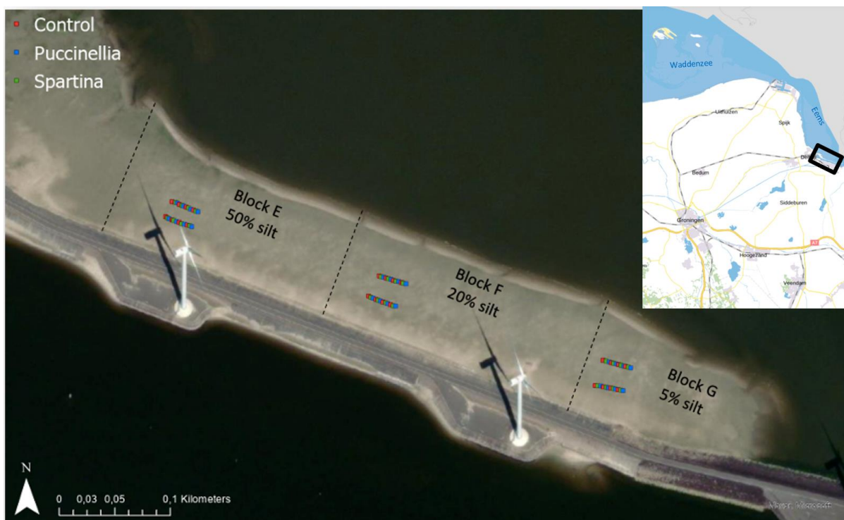
Figure 4 Satellite image of the Marconi site made with dredged material in the Ems estuary, close to the port of Delfzijl (NL). Locations of vegetation measurements are indicated in the blocks with different sediment compositions. Vegetation plots were planted at two elevations and are denoted by coloured pixels. Red pixels indicate the sample stations analysed in this study. Source: Maxar Technologies; www.satellietdataportaal.nl
