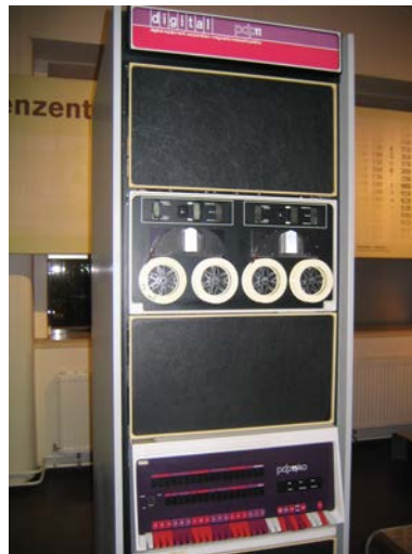
Figure 5: The Digital Equipment Corporation PDP 11/40 minicomputer which formed the core of the Nobin-Zis hospital information system (from: Wikipedia).
