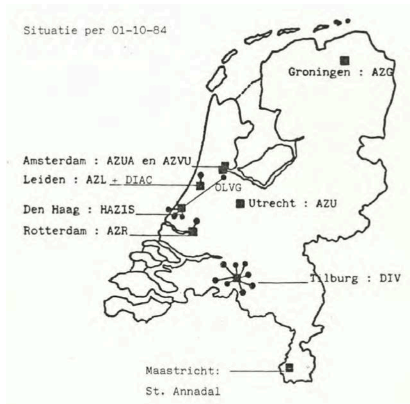
Figure 7: The BAZIS collaboration in 1984. The black squares are the hubs of the collaboration with their own computer centers. The black dots are hospitals linked with the hubs (from: Anon. (1985), Het ZIS in vogelvlucht , Leiden: BAZIS).
