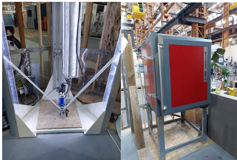
Figure 6. The 3D clay printer (left) and the kiln (right).
