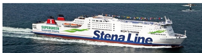
Figure 11, World's first methanol powered ship, the Stena Germanica launched in 2015 in Kiel Sweden (Portstrategy, 2015)
