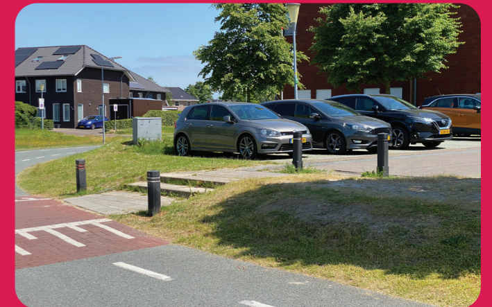
Figure 4.50: Parkingplace in Duiven that is only reachable by stairs. Makes it difficult or impossible to reach for persons with disabilities.
