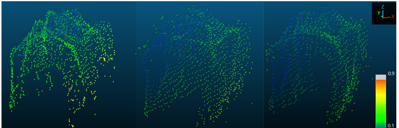
Figure 15. CWSI point cloud of plant 1 from the nadir flight (left), oblique flight (middle) and the combined flights.
