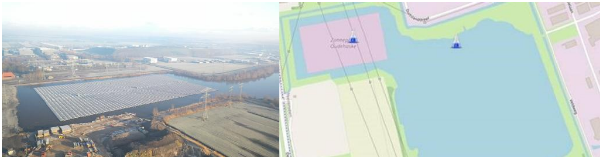
Figure 3: FPV system and sensors Oudehaske. In the left picture the part of the lake with the panels are shown. The right picture shows the entire lake with the FPV panels (pink rectangle) and the measurement locations (blue dots).
