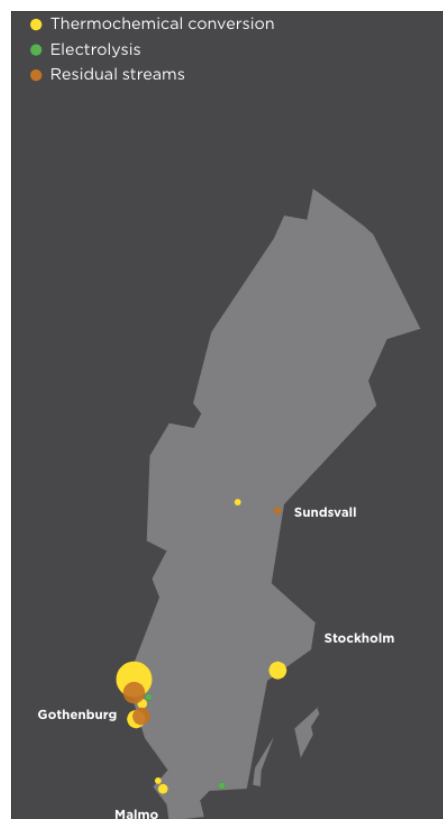
Figure 2: Schematic image of Sweden's hydrogen production and use locations (Fossil Fritt Sverige, 2021)
