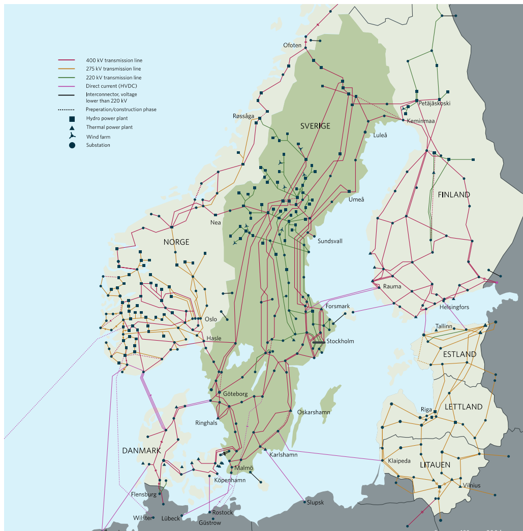
Figure 3: Visualisation of the Swedish electricity transmission network (Svenska Kraftnät, 2020b)
