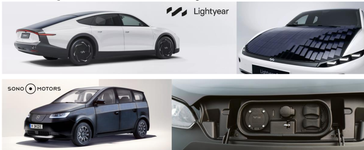
Figure 3: The Lightyear 0 has an aerodynamic exterior silhouette with large roof surface for VIPV yield optimization and grid-independency, while the Sono Sion has three types of sockets for DES optimization and grid-symbiosis (Lightyear, 2023b; Sono Motors, 2022).
