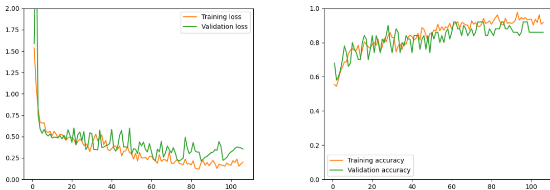
Fig. 17: Typical example of training and validation performance per epoch when training the REM model. The model shows to have some difficulties generalizing to the validation set.
