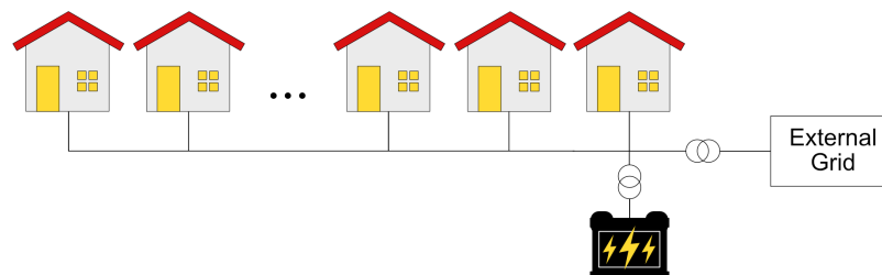
Figure 3.1: Schematic overview of the synthetic electric grid with a variable number of households.
