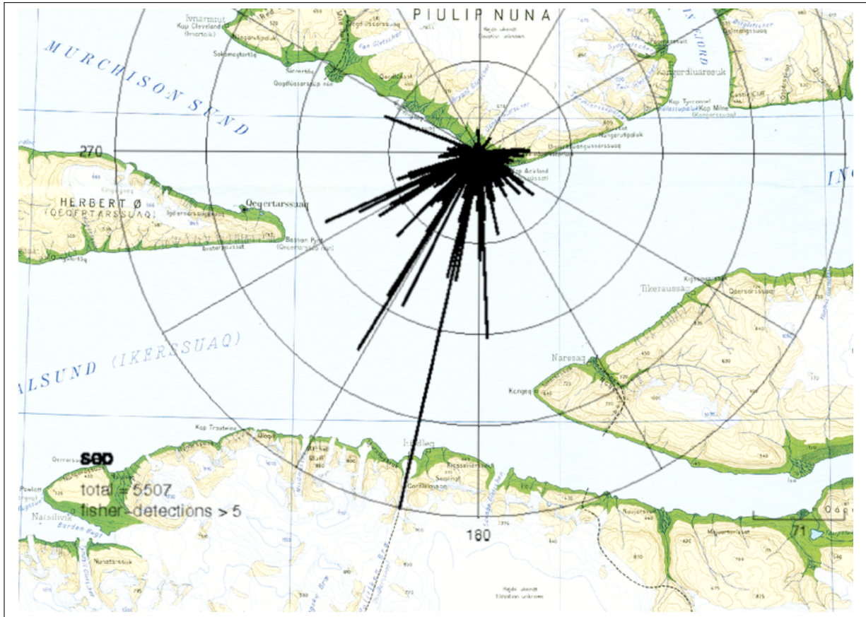
Figure 4.9: Rose-diagram showing the distribution of the strong events, i.e. Fisher ratio higher than 5, detected for the months September. For every back-azimuth degree, the number of detections is counted. The total number of detections displayed in the rose diagram is 5507 ( \sim 18\% of all detections) and the longest bar corresponds to a maximum of 232 detected events from a direction of 192^\circ - 193^\circ .
