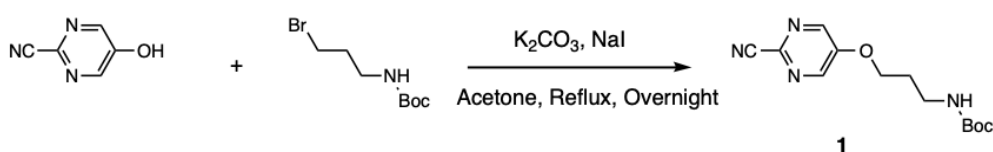
Scheme 1. Reaction scheme for introduction of Boc protected amine.
