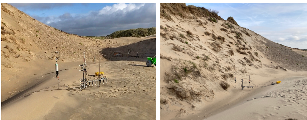
Figure 3.7 Position of northern SalDec and Sonic Anemometer. Left: on the hills next to the gully on day 5, right: in the northern gully on day 7.
