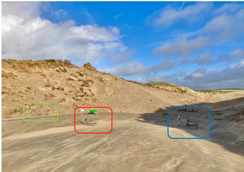
Figure 3.5: Set-up of the three SalDecs and sonic anemometers as they were positioned most days. Photo was taken on day 5.
