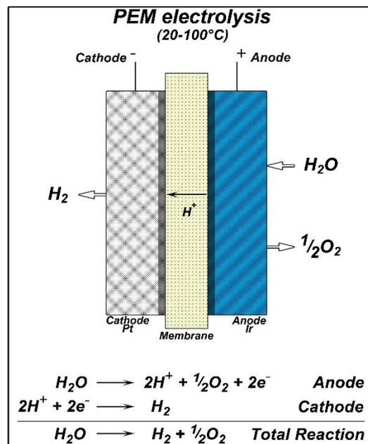
Figure 9 - Schematic visualization of PEM electrolyzer
