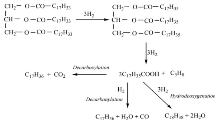
Figure 23 - Conversion of triglycerides to alkanes (Sotelo-Boyás et al., 2012)
