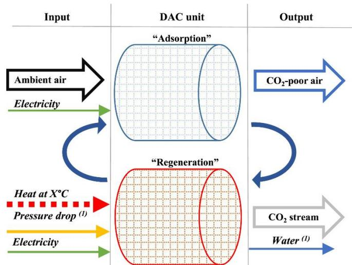
Figure 8 – Schematic visualization of LT DAC operation (Fasihi et al., 2019)
