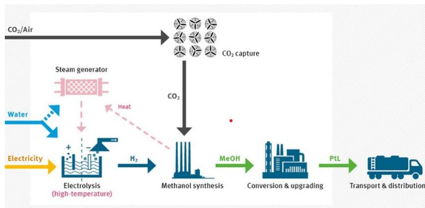
Figure 10 - Production route of e-fuels through methanol synthesis (German Environment Agency, 2016)
