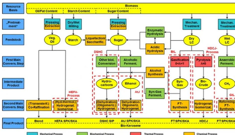
Figure 6 - Overview of conversion processes from biomass feedstock to bio-SAF (Neuling & Kaltschmitt, 2015)
