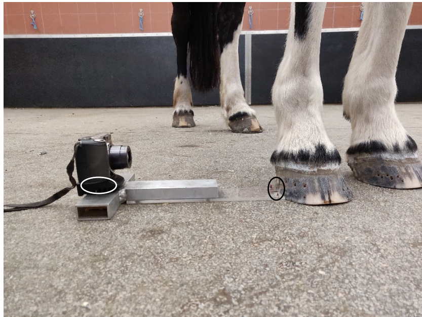
Figure 4: the camera construction; level (highlighted with the white circle) and pins (highlighted with the black circle), for the hoof pictures.
