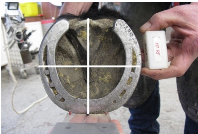
Figure 9: solar view of the right front hoof of horse 2 in week 7 with steel shoes. The wear distribution of the shoe in the four regions was classified with the help of the scale for wear of the shoe mentioned above. Medial heel: I, lateral heel: III, medial toe: II, lateral toe: IV.
