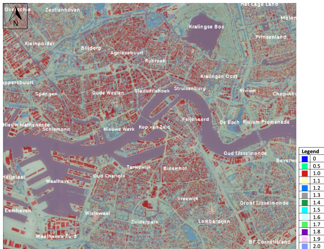
Figure 19: Change in the spatial pattern of the PET between PET calculation on summer day with a return period of 33 years and 1 year in Rotterdam. (Scale 1:100,000)
