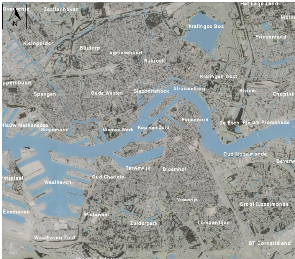
Figure 24: Shaded areas in current climate and spatial conditions in Rotterdam, the Netherlands for June 21 st at 14:00. Darker areas are shaded and lighter areas are not shaded. (Scale 1:100,000)
