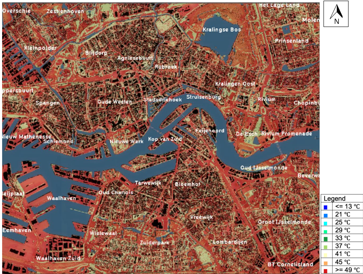
Figure 9: PET in Rotterdam on a hot summer day with a return period of 33 years. Model run 1.1 (Scale 1:100,000)
