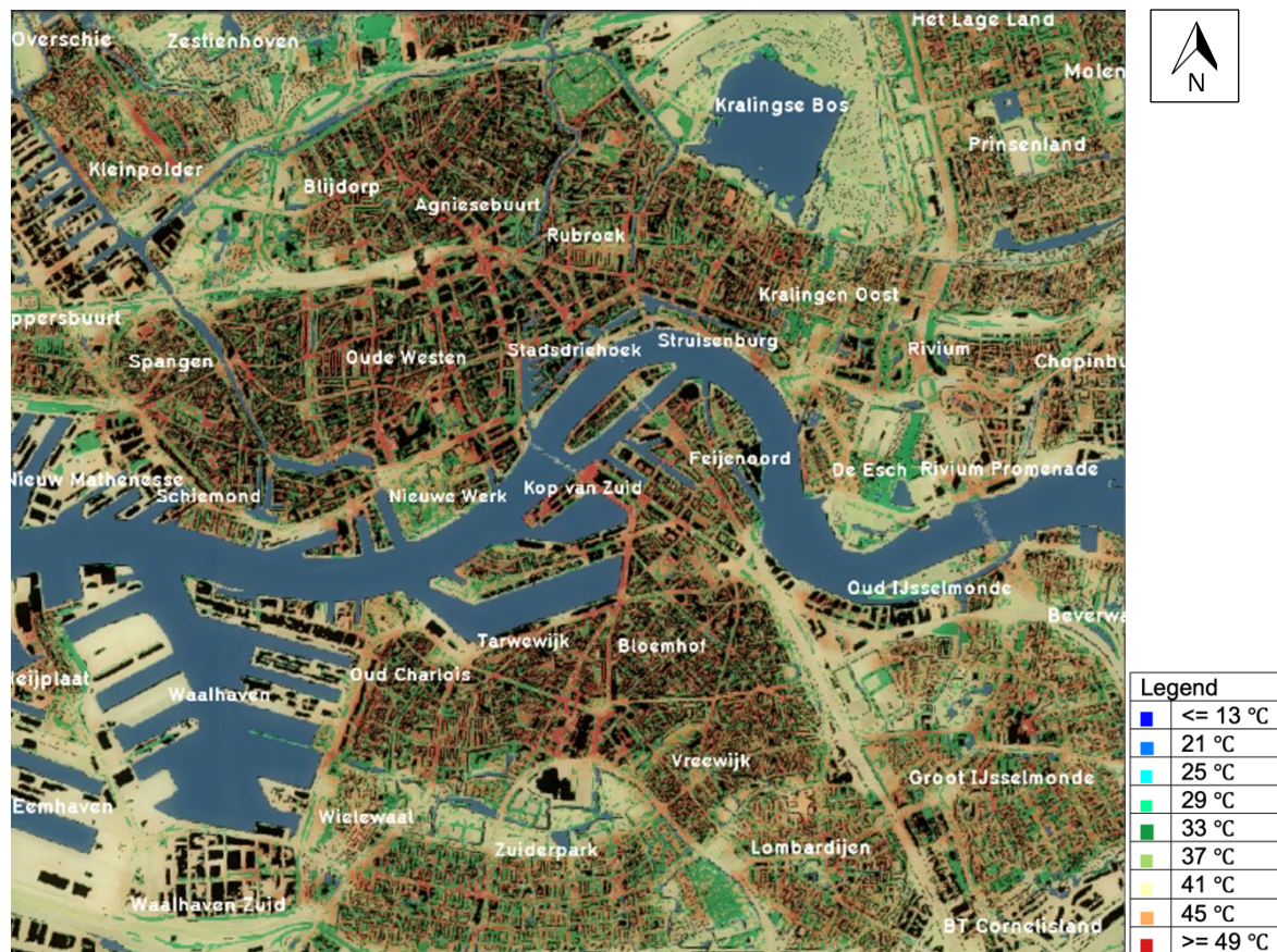
Figure 16: PET in Rotterdam on a summer day with a maximum daily temperature with a return period of 1 year. Model run 1.4 (Scale 1:100,000)
