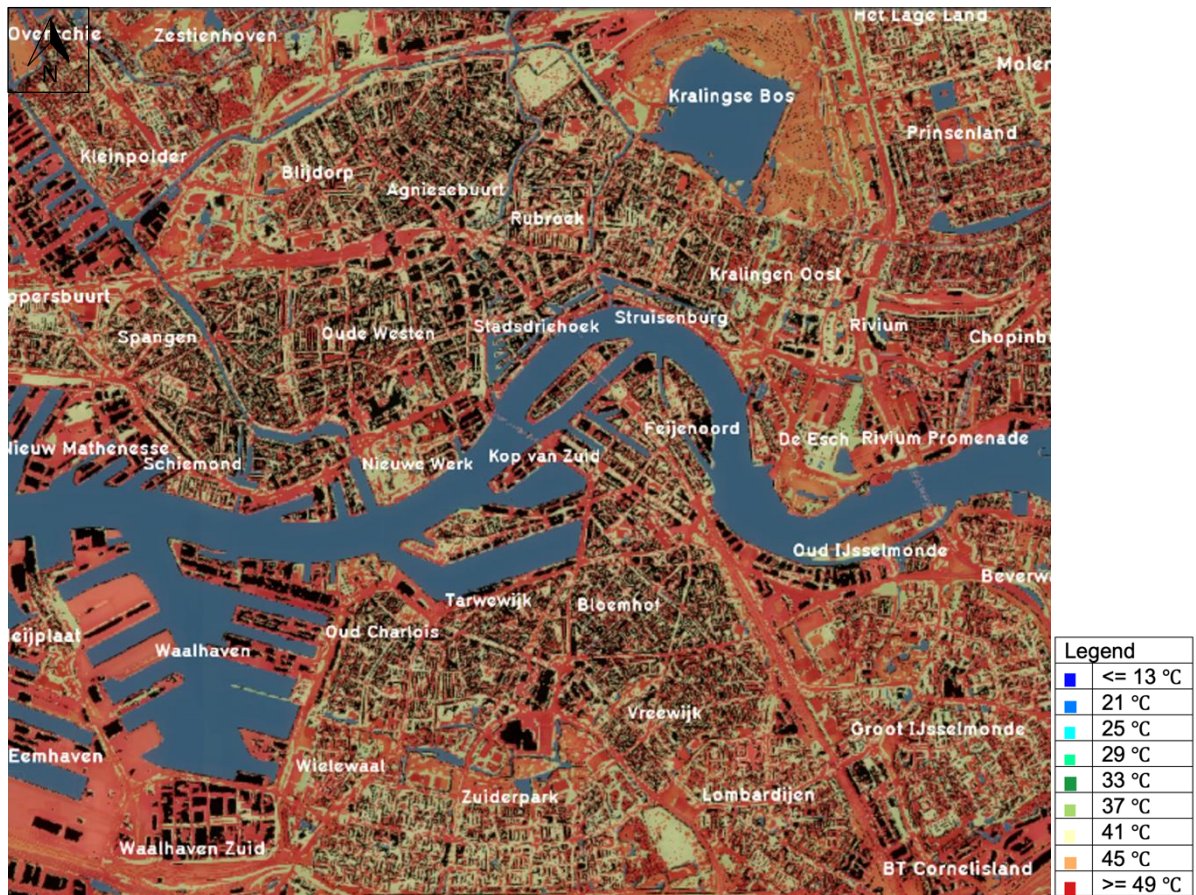
Figure 27: Forecasted PET on a hot day with a maximum daily temperature with a return period of 3 years in Rotterdam in 2050 for the W_H -climate change scenario. Model run 2.1 (Scale 1:100,000)
