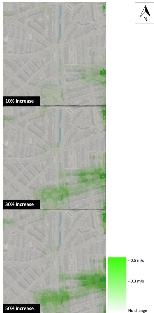
Figure 52: Difference in wind speed for model runs with different increases in number of trees, compared to the original number of trees. Green areas indicate a decrease in wind speed. The brighter the green, the more the wind speed decreases as a result to the increase in trees. (Scale 1:25,000)
