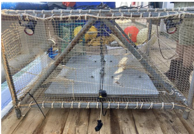
Figure 8: GoPro and bamboo stick with bait attached to the bottom of the cage, and two LetonPower lights attached right and left to the top of the cage.
