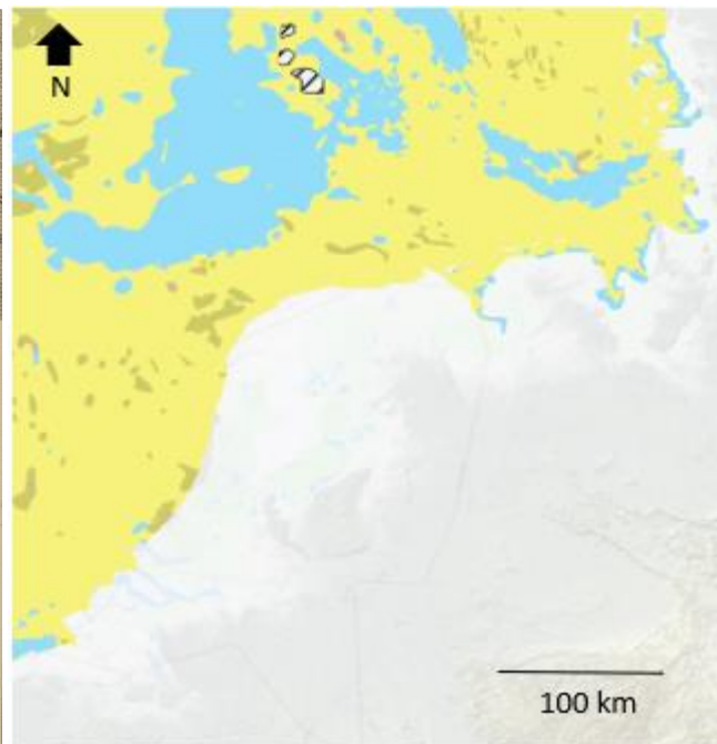
Figure 2: Map of North Sea seabed substrate today (EMODnet Geology, z.d.). Blue: mud to muddy sand; yellow: sand; dark yellow: coarse substrate; pink: mixed sediment; white and black: no data available.
