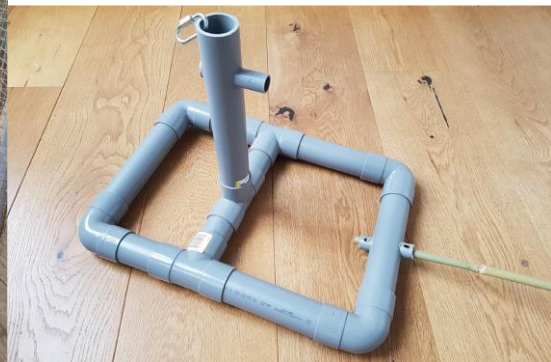
Figure 9: Frame of PVC pipes with bamboo stick to attach bait on the right and smaller pipe through the vertical pipe to attach the camera.
