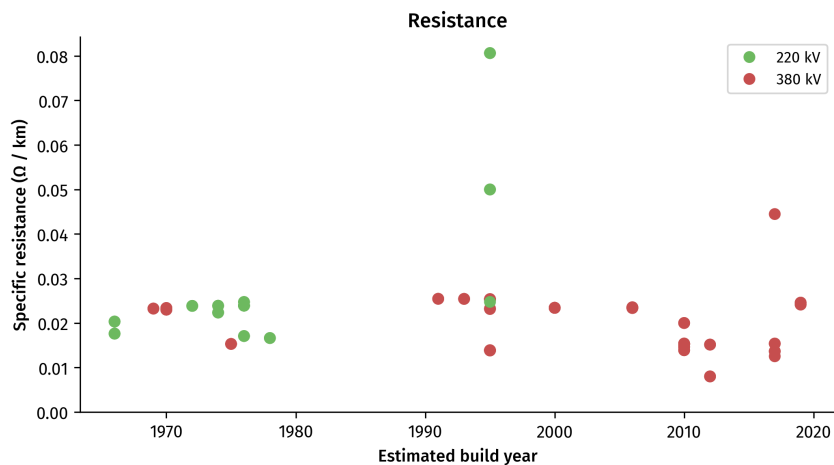
Figure A.1: Plot of the specific resistance of transmission lines against the (estimated) build year of the line. Based on data from TenneT (2023).
