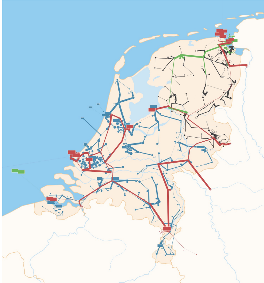
Figure 4.17: Result of solving the optimal power flow for 2020. Node sizes are proportional to their load or generation, and widths of the edges are proportional to the amount of power transported over that edge. In the solution, not all the power generated by a plant is always transported over a line, when this is not required to satisfy the loads. This is the reason some power plants look to be disconnected while still producing electricity.
