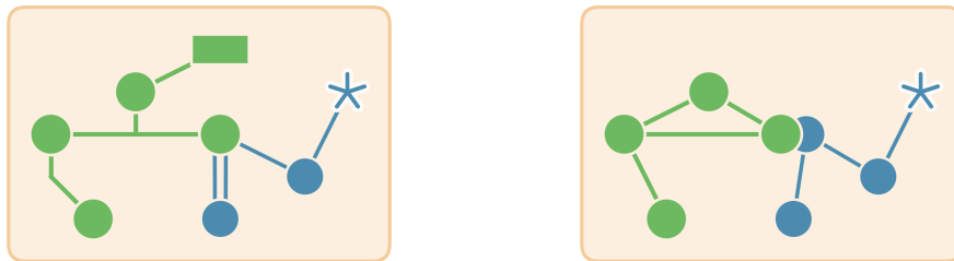
Figure 3.4: Example of a network (left) and its reference version (right). Creating a reference version ensures that calculations on networks from different sources can be compared to each other. The colors indicate different voltage levels, the rectangle is a power plant, and the star symbol is a foreign subnet. Between the overlapping nodes is a transformer.
