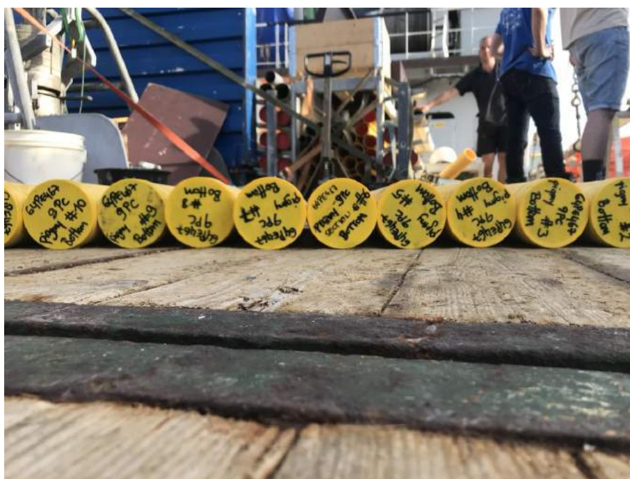
Figure 14. Sections of the piston core collected from the Pigmy Basin (Station 9).
