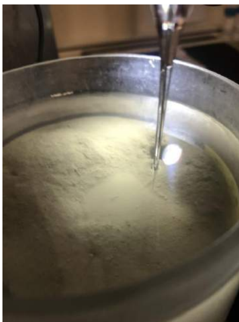
Figure 13. Micro-electrode used for O 2 profiling
