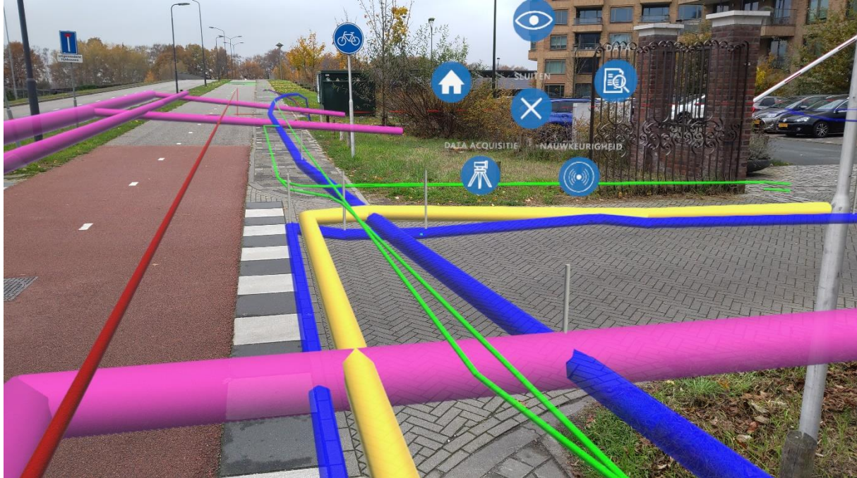
Figure 50: Better perspective in AR with vertical reference features.
